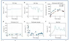
Liver performance parameters during ex situ normothermic machine perfusion
