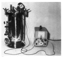
The hyperbaric chamber and perfusion. The perfusion tubing is slotted in the pump head and connected to the inflow and outflow nipples on the chamber wall. The pressure gauge, safety valve, quick-coupling Connector, exhaust valve, and thermometer are visible on the chamber. (From Ackermann et al BJS 1966)
